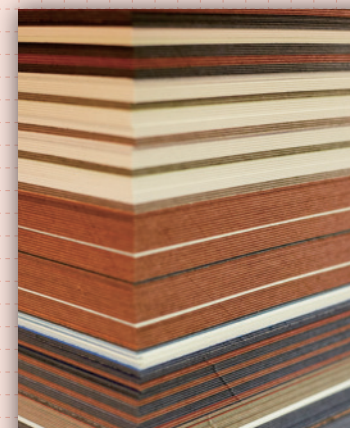
Vulcanized fiber as a material. There are many types of colors and thicknesses.
